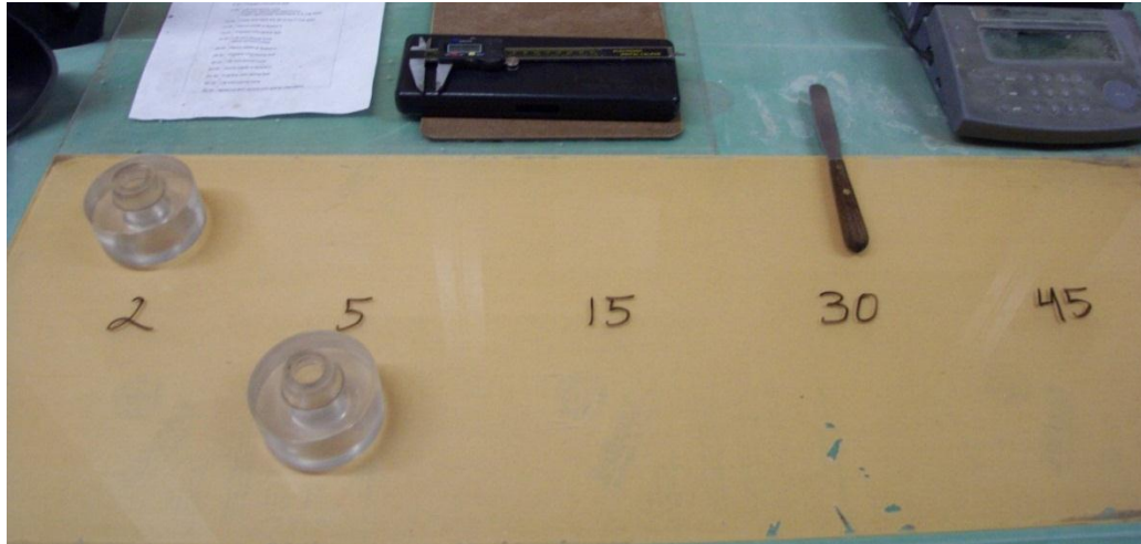
Figure 4.10 – Miniature slump cones and equipment
