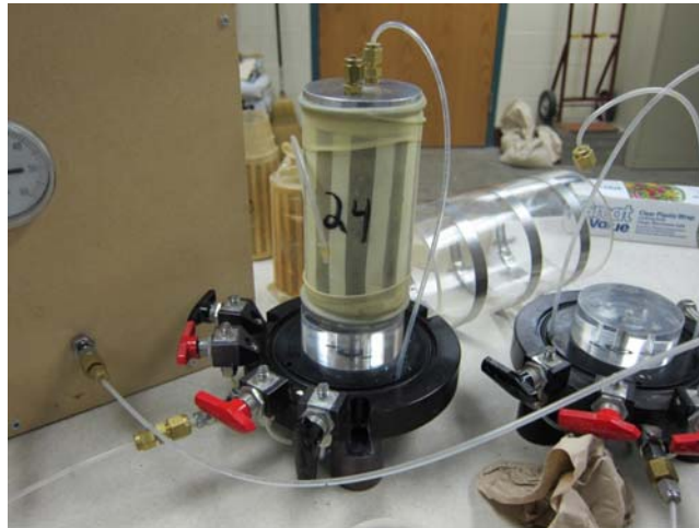
Figure 24 – Specimen after testing placed in pressurized triaxial cell
