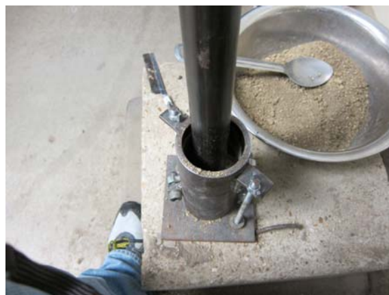
Figure 11 – Compaction of one layer in the 2.9"-dia. mold
