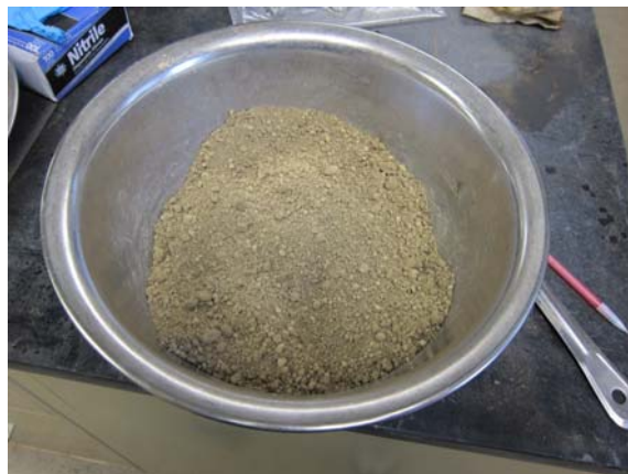
Figure 9 – Soil and additive after mixing
