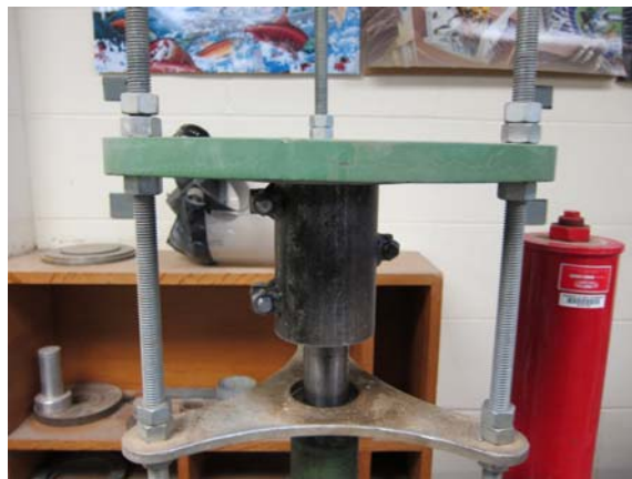
Figure 13 – Compaction mold inserted into extrusion frame
