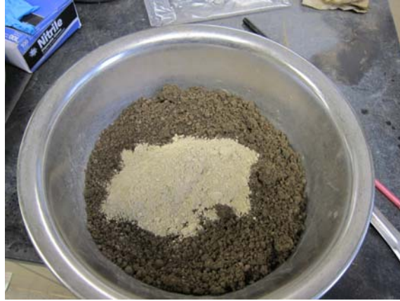
Figure 8 – Soil and additive combined prior to mixing
