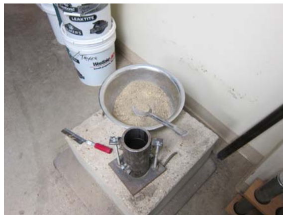
Figure 10 – Compaction equipment and soil
