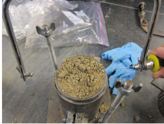
Figure 12 – Trimming of excess soil after compaction
