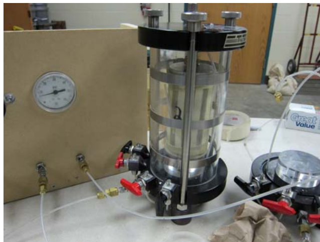
Figure 25 – Sample confined in pressurized cell
