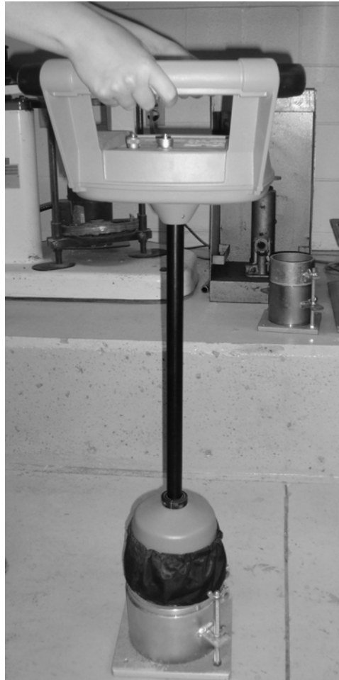
Figure 27 – BCD testing on a compacted soil sample in a 6 inch split mold
