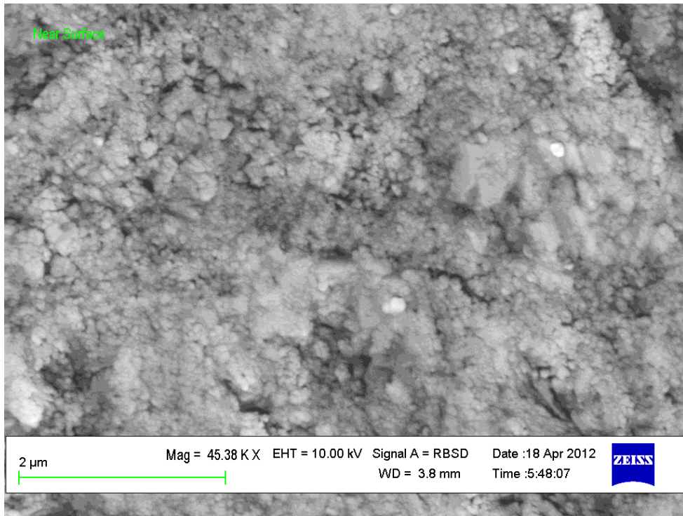
Figure 30: Micron scale structure of the mortar paste near the surface of Chlorinated Rubber MFCC treated concrete
