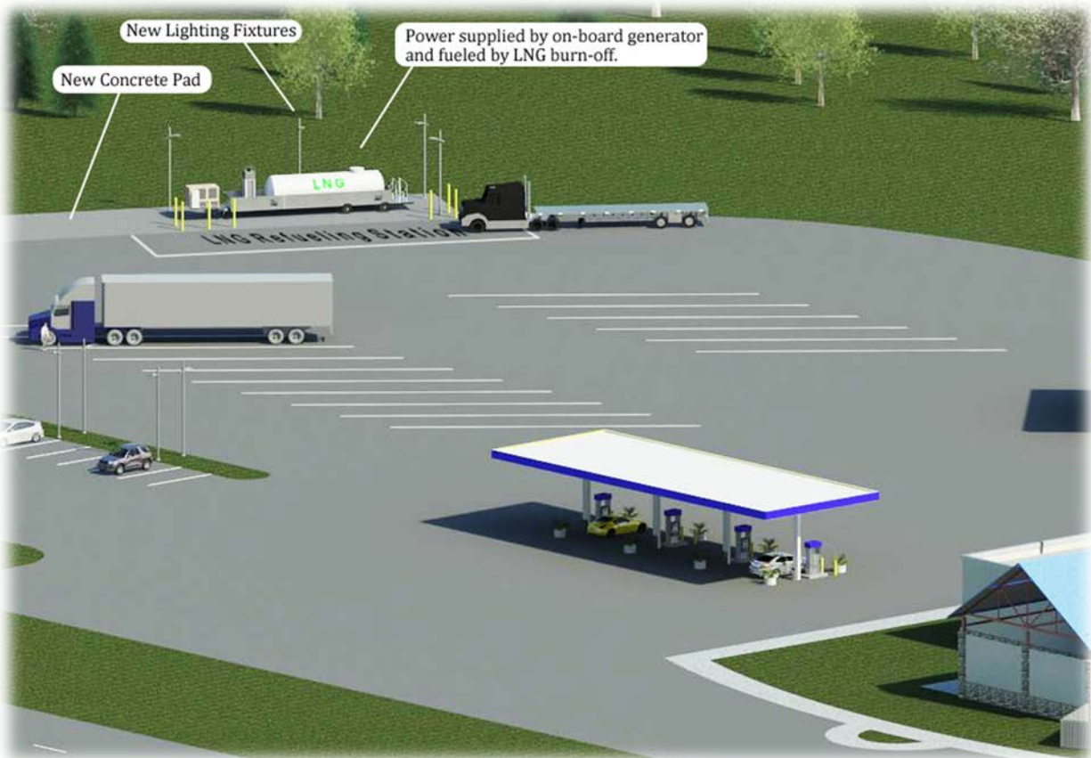
Figure 3.19. Proposed installation of an LNG mobile fueling station at an existing service plaza. Note the reduced physical space and level of infrastructure to implement this option
