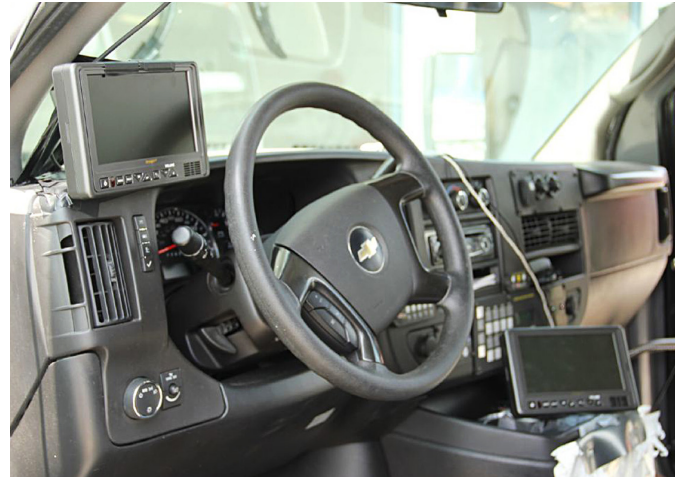
Monitors for left and right side view cameras were placed next to the steering wheel at 10 and 4 o'clock.
