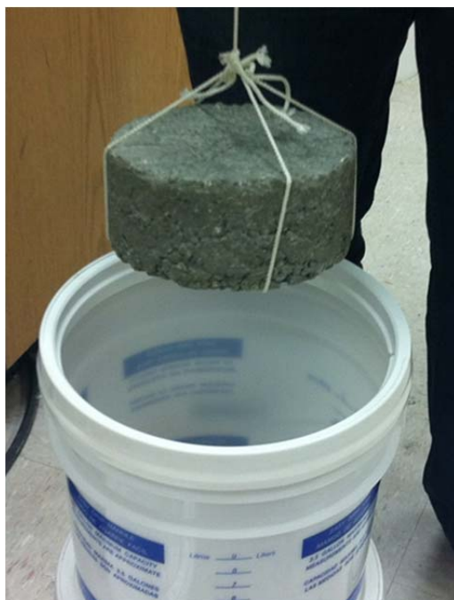
Figure 7: Monolith Suspended from the Lid of Gamma Seal ® by Nylon Cord
