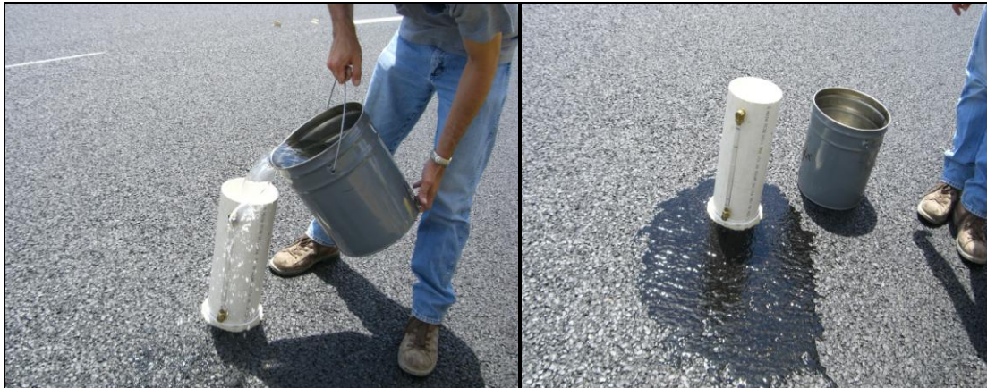
FIGURE 3 Test Method Tex-246-F, Field Water Flow Test.
