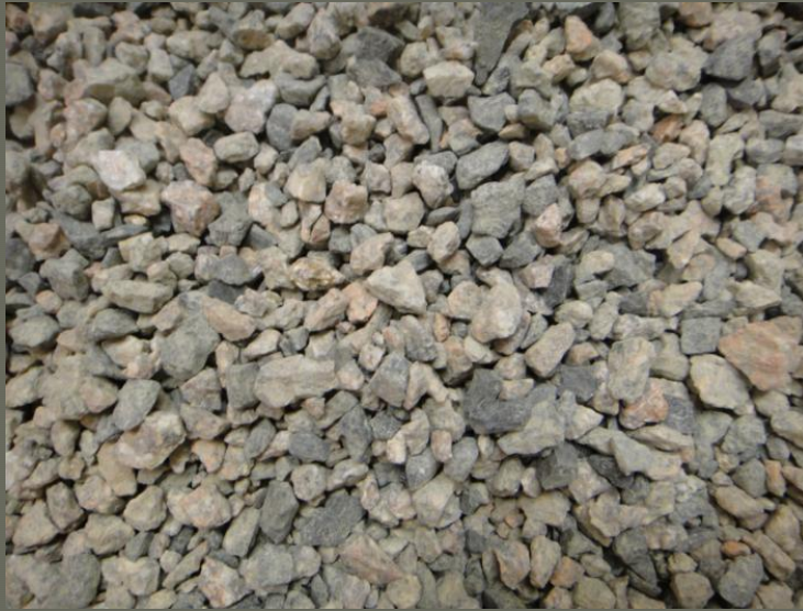
Mill Creek Aggregate (1/4-in chips) used by APAC at Dallas HMA Plants
