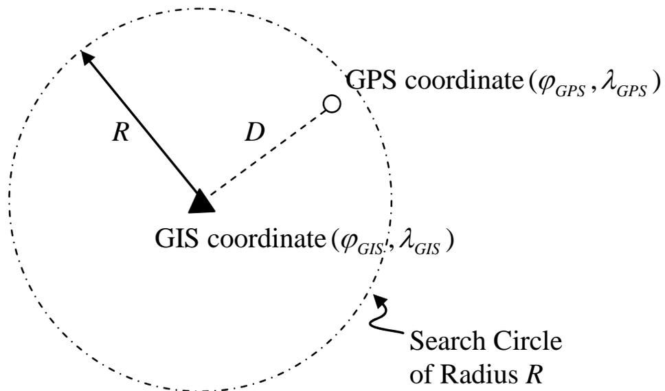
Figure 4. Quantitative Position Validation Procedure
