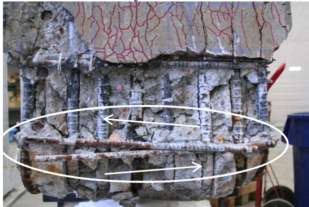
(e) Anchorage debonding of transverse U-bars
