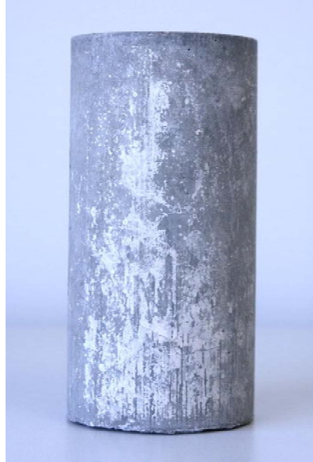
(a) Cured concrete cylinder (with hairline cracking)
