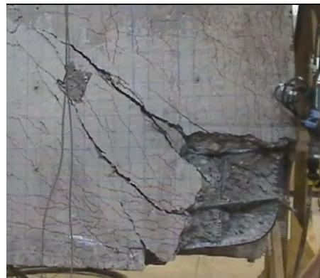
(c) Singly reinforced beam (after failure)
