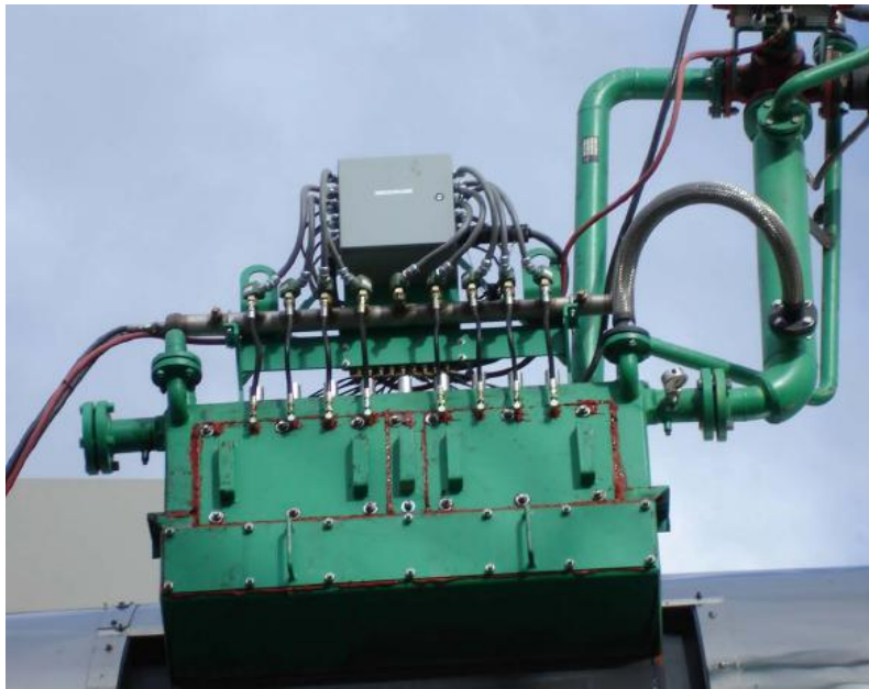
Figure 3.4: Multi-Nozzle foaming device (after Astec, Inc.).
