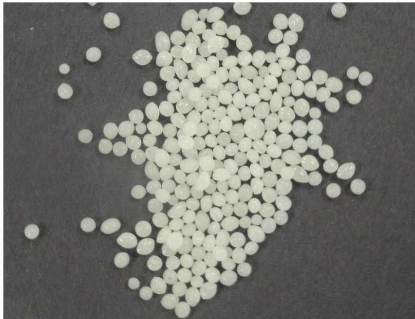
Figure 3.3: Sasobit WMA Additive
