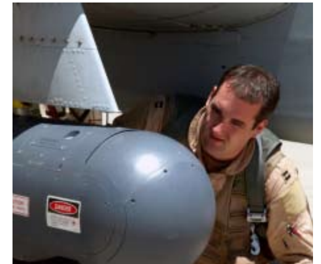
An A-10 pilot checks his Litening Precision Targeting pod before a mission in Afghanistan
