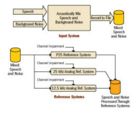
The tests compare digital and analog communications technology in laboratory simulations of public-safety communications environments (see graphic). Atkinson said that speech and noise from such environments will be tested in a manufacturer-independent manner using reference communication systems.
