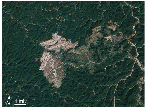
The Hobet coal mine in West Virginia is pale tan against the dark green forest. The pale green areas near the mine are reclamation areas where plants are beginning to grow. Landsat images like this one from September 2012 are used to monitor surface mines and reclamation efforts.
