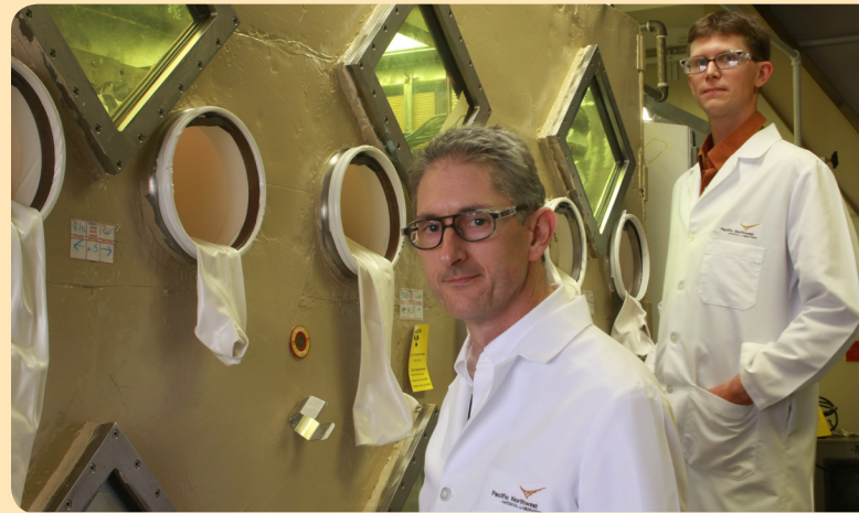
Researchers design, build and operate small-scale radiochemical process test equipment in gloveboxes.
