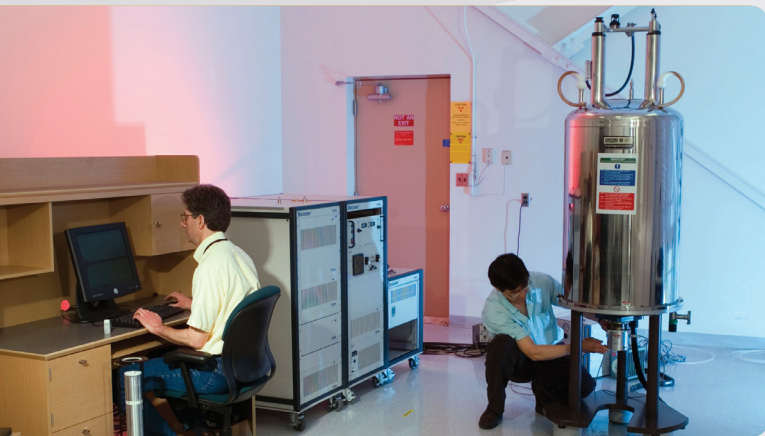
The RPL's Radiological NMR Laboratory houses a 300-MHz spectrometer and a variable field spectrometer.
