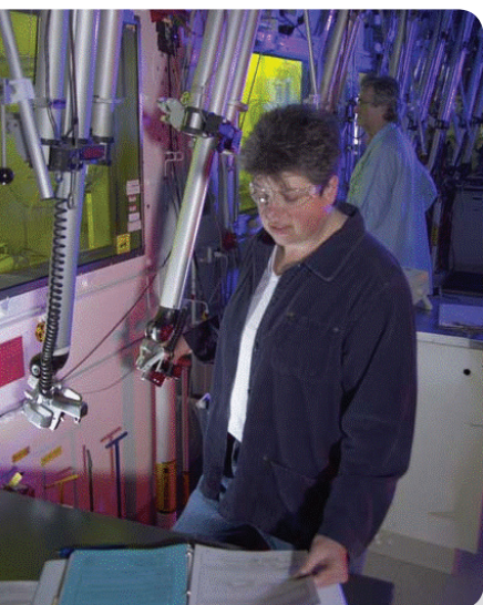
Researchers at the RPL conduct analytical research on nuclear materials using hot cells that shield the researcher from the radiation.
