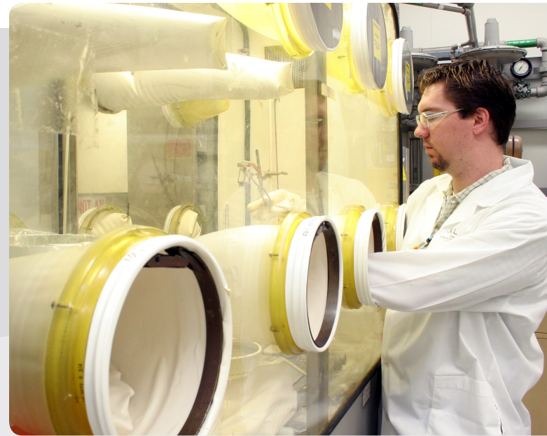
One of the unique capabilities of the RPL is actinide research. Here, a researcher works with a plutonium sample using one of several gloveboxes in the RPL.
