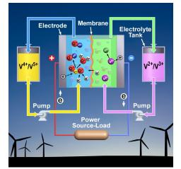
This artist's rendering of an upgraded vanadium redox battery shows how using both hydrochloric and sulfuric acids in the electrolyte significantly improves the battery's performance and could also improve the electric grid's reliability and help connect more wind turbines and solar panels to the grid.
