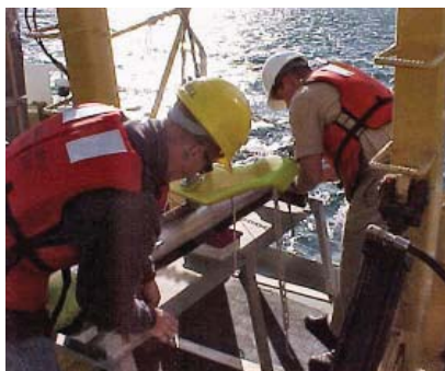
Deck crew lowers side-scan sonar "fish"
