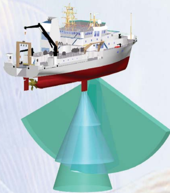
The ship is equipped with multiple sonar systems to meet its missions.
