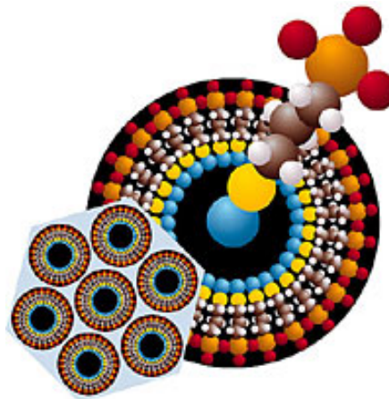
Shown is a SAMMS™, which forms effective sorbents for a wide variety of species including mercury, heavy metals, radionuclides and anions.
