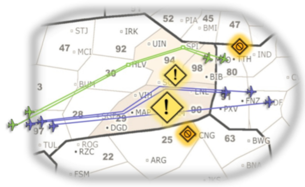
Figure 1. Flow-based trajectory management operations adjust traffic flows in response to local area constraints or disturbances (e.g., traffic congestion, convective weather), by modifying the trajectories of aircraft that are already in flight. A NextGen “best-equipped, best-served” policy for rewarding early adopters of key new technology can be used to determine who should receive priority access to constrained airspace (blue aircraft).
