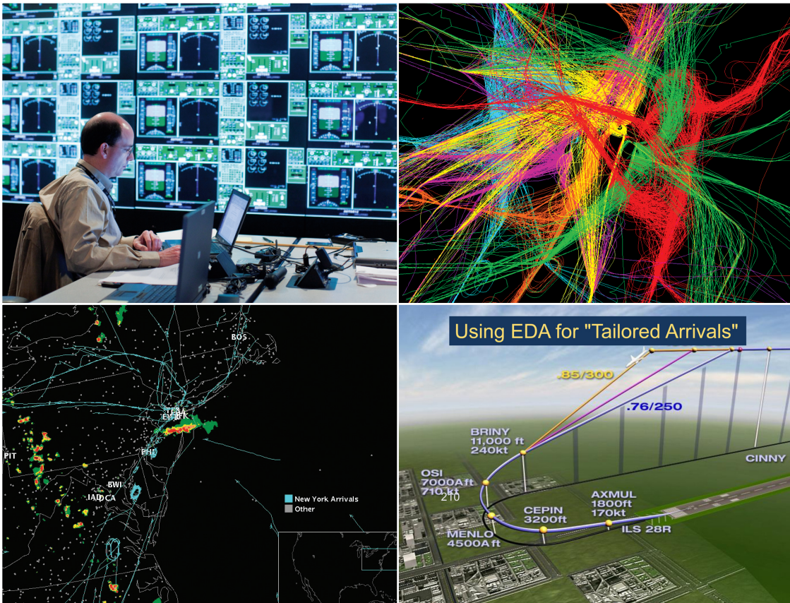
Images (Clockwise, left to right) Air Traffic Operations Laboratory: This lab, which also includes human-piloted simulators, supports research into ways to improve aircraft separation and resolve potential aircraft conflicts. Metroplex Operations: Simulations of arrivals and departures at airports close to each other, such as in New York City, help find solutions for reducing delays but increasing capacity. Efficient Descent Advisor: NASA is working on tools to help air traffic controllers make approaches and descents more efficient while also avoiding conflicts with other aircraft. Tools for Reducing Weather Delays: Developing sophisticated computer algorithms that reduce delays and reroutes caused by bad weather, especially approaching busy airports like those near New York City, is a key focus.
