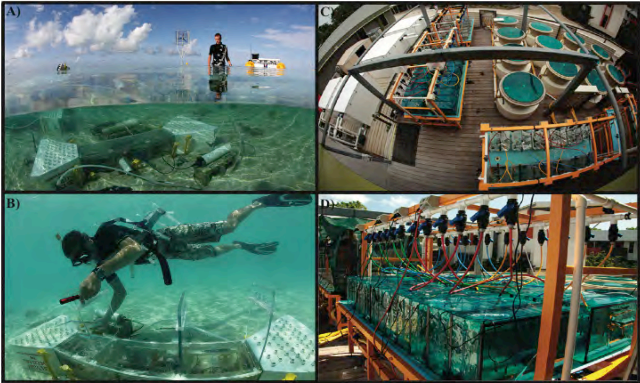
Figure 1: Coral reef climate change experimental systems on Heron Island, Great Barrier Reef, Australia. In A) the Coral Proto – Free Ocean Carbon Enrichment System (CP-FOCE), an in-situ ocean acidification system currently deployed on the reef flat at Heron Island. The system uses a system of integrated instruments connected to four experimental chambers to control the pH in the chambers as an offset from the environmental pH using a float that has a series of computer pods that determines the rate and direction of dosing. The doors in the chambers are closed regularly B) for calcification and respirometry measurements. In C) the pCO 2 -stat and temperature climate change system is shown. Each of the 4 large white boxes are 8,000 L insulated sumps that are each controlled to a different environmental scenario of pCO 2 stat system and large heater-chillers. The manipulated water from each of these sumps is then pumped to three replicate, 300 L mini-reefs (12 total) with Lee filters stimulating the 5 m water depth where the reef organisms were collected. The treatment water is also pumped to 3 experimental tables D) which can hold a total of 72, 30 L glass aquaria fitted with LEE filters to stimulate the light environment where the organisms were collected.
