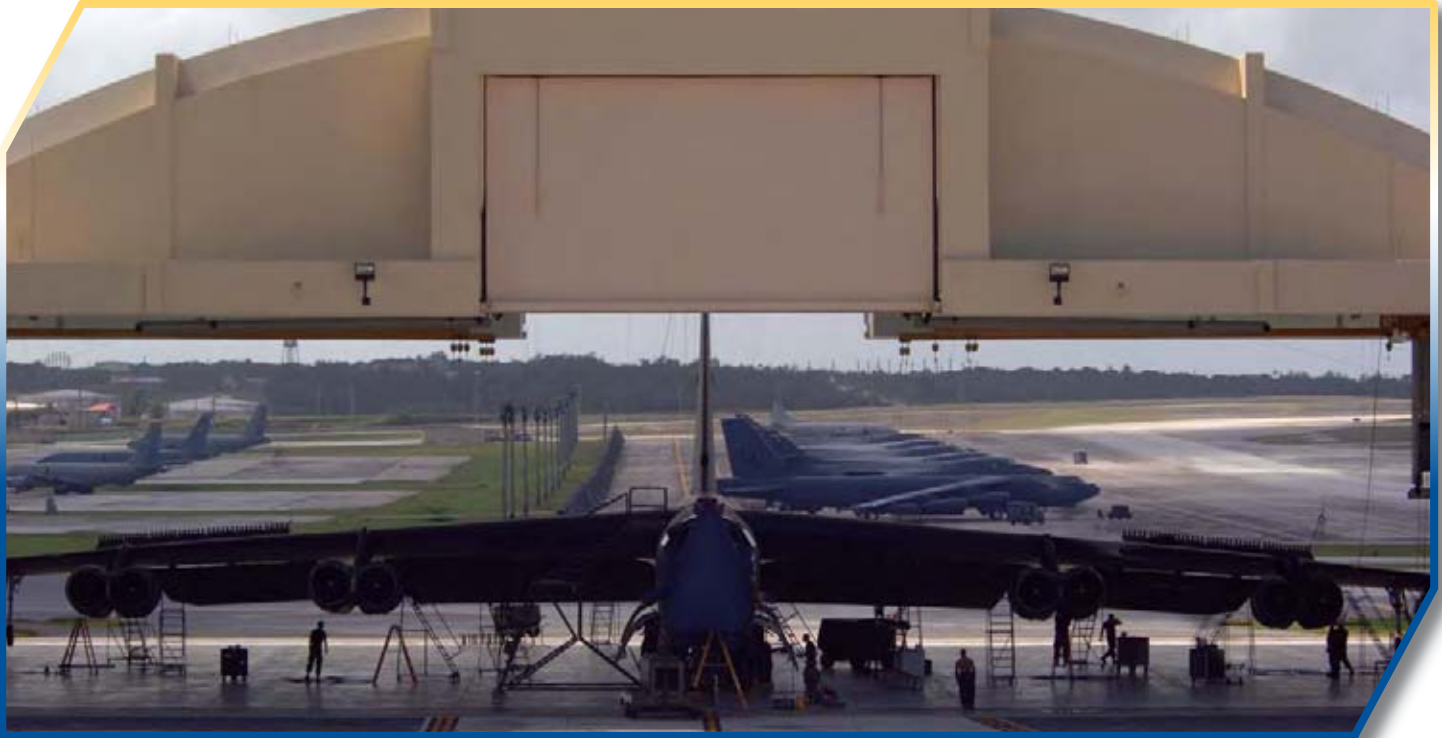
B-52 Stratofortress mechanics inspect their aircraft during phase maintenance at Andersen AFB, Guam. The B-52s come here from a forward-deployed location and go into phase maintenance after 300 flying hours. The hangar can house any type of Air Force aircraft. (U.S. Air Force photo by MSgt Val Gempis)
