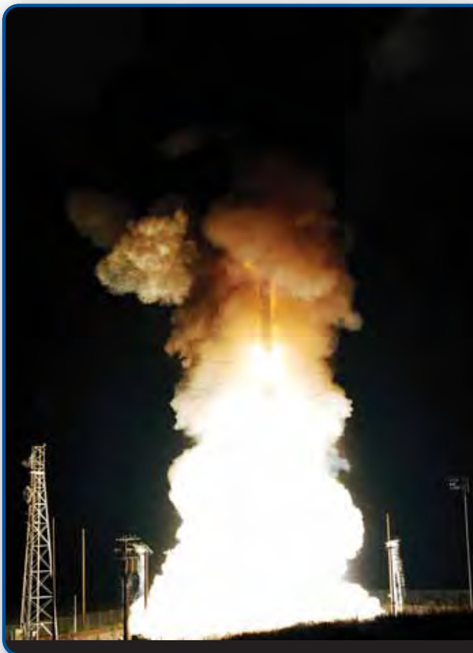
A Minuteman III intercontinental ballistic missile successfully launches from North Vandenberg AFB. The missile was configured with a National Nuclear Security Administration (NNSA) test assembly in which three unarmed re-entry vehicles traveled approximately 4,190 miles to their pre-determined targets.
