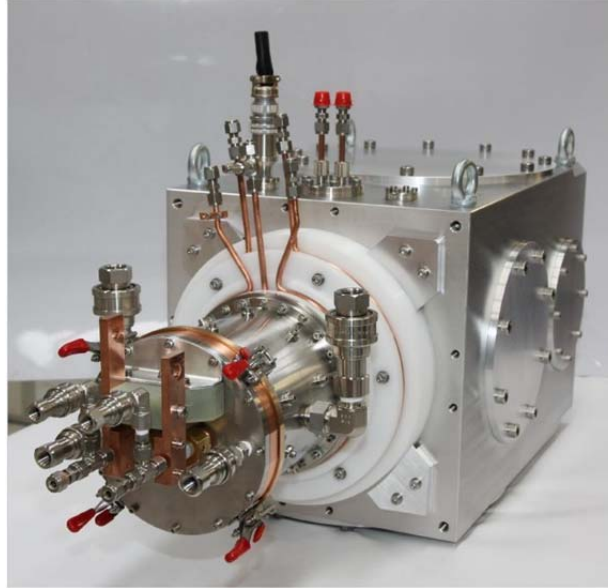
Figure IV-1: Photograph of the D-Pace ion source (foreground) with the vacuum chamber.
