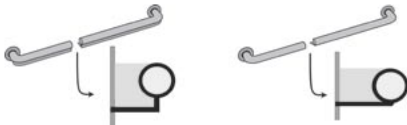
Profiles of accessible grab bars with suicide prevention feature.
