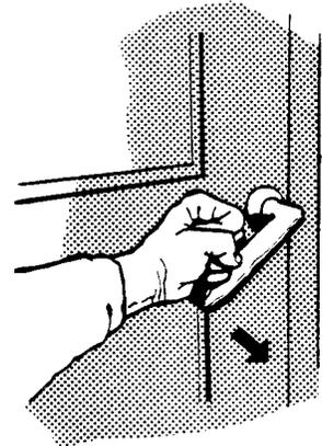
wrist to operate. Lever-operated mechanisms, push-type mechanisms, and U-shaped handles are acceptable designs. When sliding doors are fully open, operating hardware shall be exposed and usable from both sides. Hardware required for accessible door passage shall be mounted no higher than 48 in (1220 mm) above finished floor.
