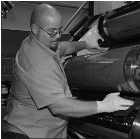
David Thornton, Simultan Pressman, mounting plate for printing.
