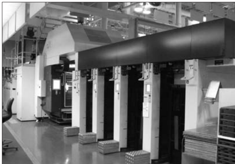
As part of the Bureau's retooling effort, two new intaglio currency presses were installed in WCF.
