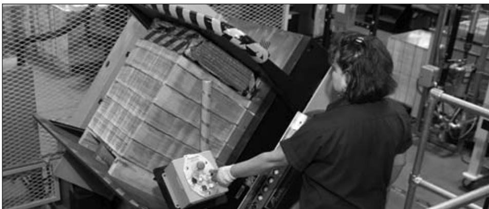
Samnieng "Sammy" Ruiz operates a mechanized jogger/aerator that separates the sheets of currency paper in preparation for further processing. This equipment eliminates the need for manual jogging and restacking which reduces repetitive motion and heavy lifting injuries.
