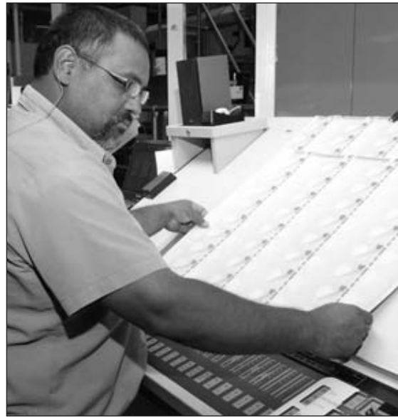
Marcus Alegria, Simultan Pressman, performing a quality review of an offset printed currency sheet.
