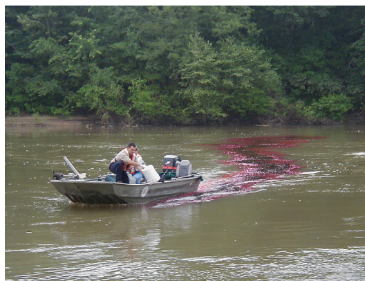
Figure 5. Injecting dye while boating across a stream (photograph by U.S. Geological Survey).
