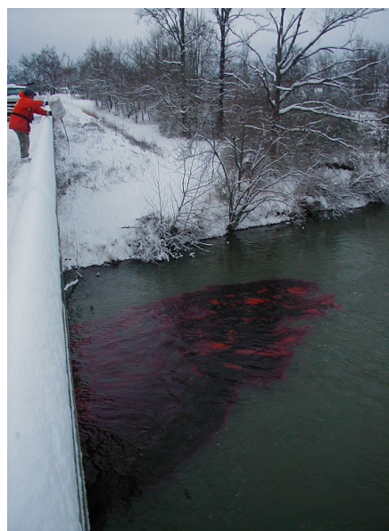
Figure 6. Injecting dye into a stream from a bridge (photograph by U.S. Geological Survey).
