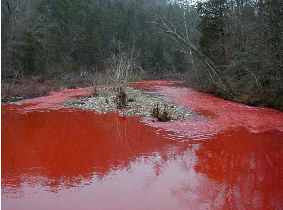
Figure 7. Lateral mixing of Rhodamine WT dye (photograph by U.S. Geological Survey).
