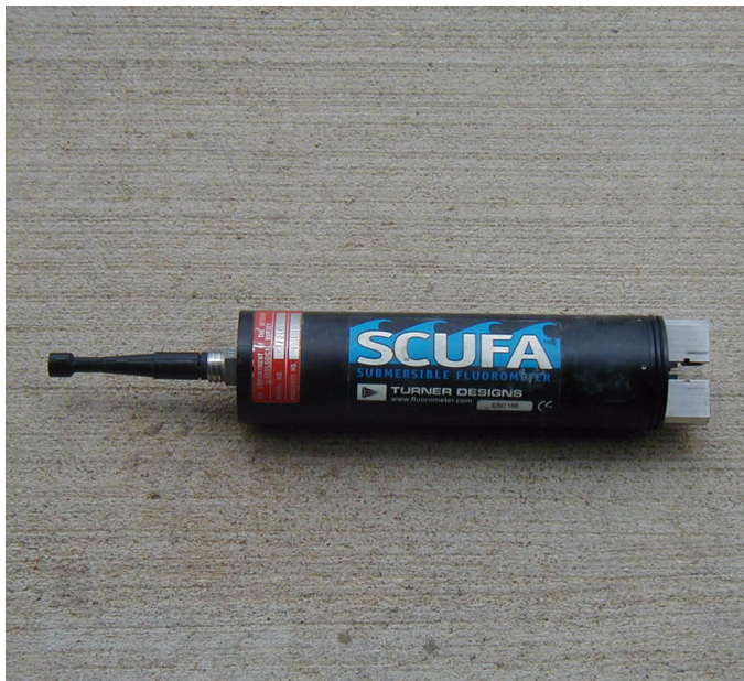
Figure 8. Self-Contained Underwater Fluorescence Apparatus (SCUFA).
