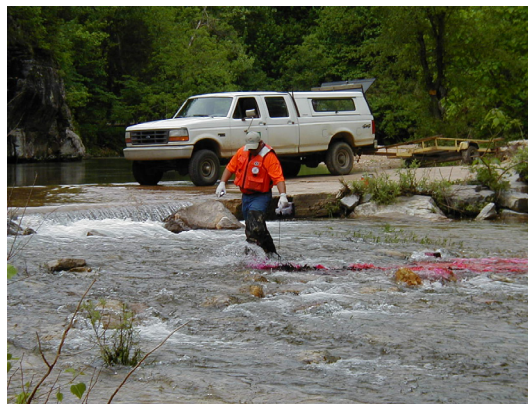
Figure 4. Injecting dye while wading across a stream (photograph by U.S. Geological Survey).
