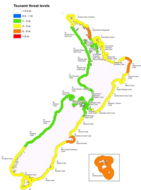
Exercise Tangaroa 2010 tsunami threat level map: The colours correspond to the maximum expected water elevation (i.e. zero-to-peak) at the coastline in metres above sea-level.
