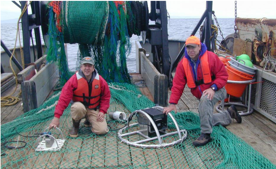
Scientists developed new underwater camera systems that can help commercial trawl fisherman adjust their nets in real-time to reduce or avoid bycatch.
