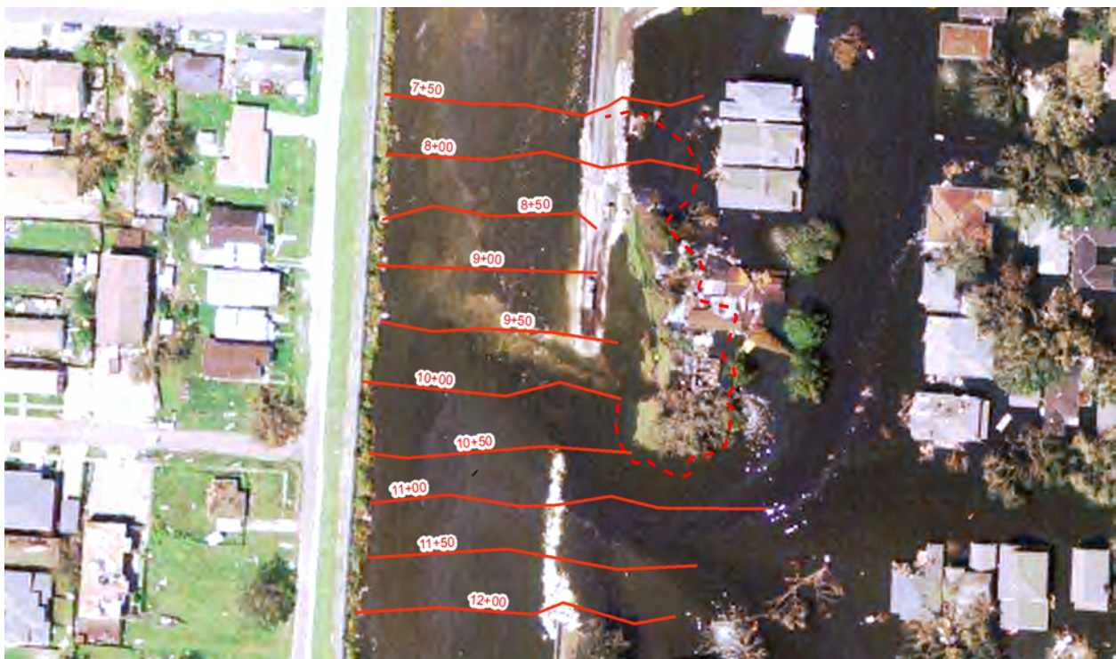
Figure VI-4. Location of multi-beam sonar survey cross-sections
