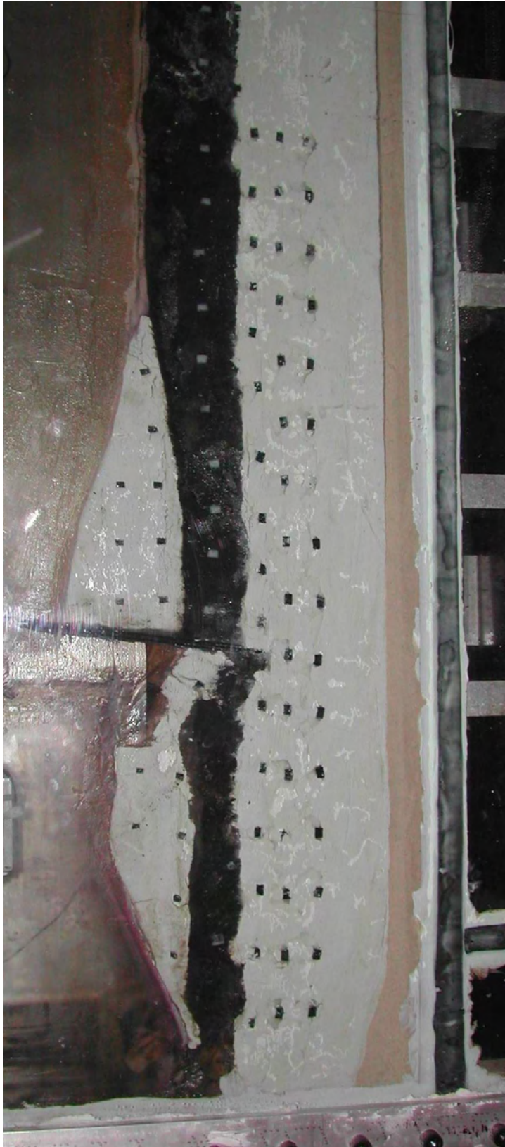
Figure VI-21. Sliding movement of the levee landward (to the right) observed at the completion of the 17th Street trial model test
