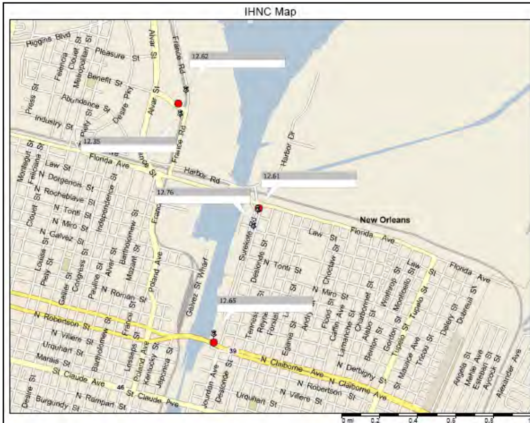
Figure III-13. Selected Post-Katrina Elevations on IHNC Floodwalls
