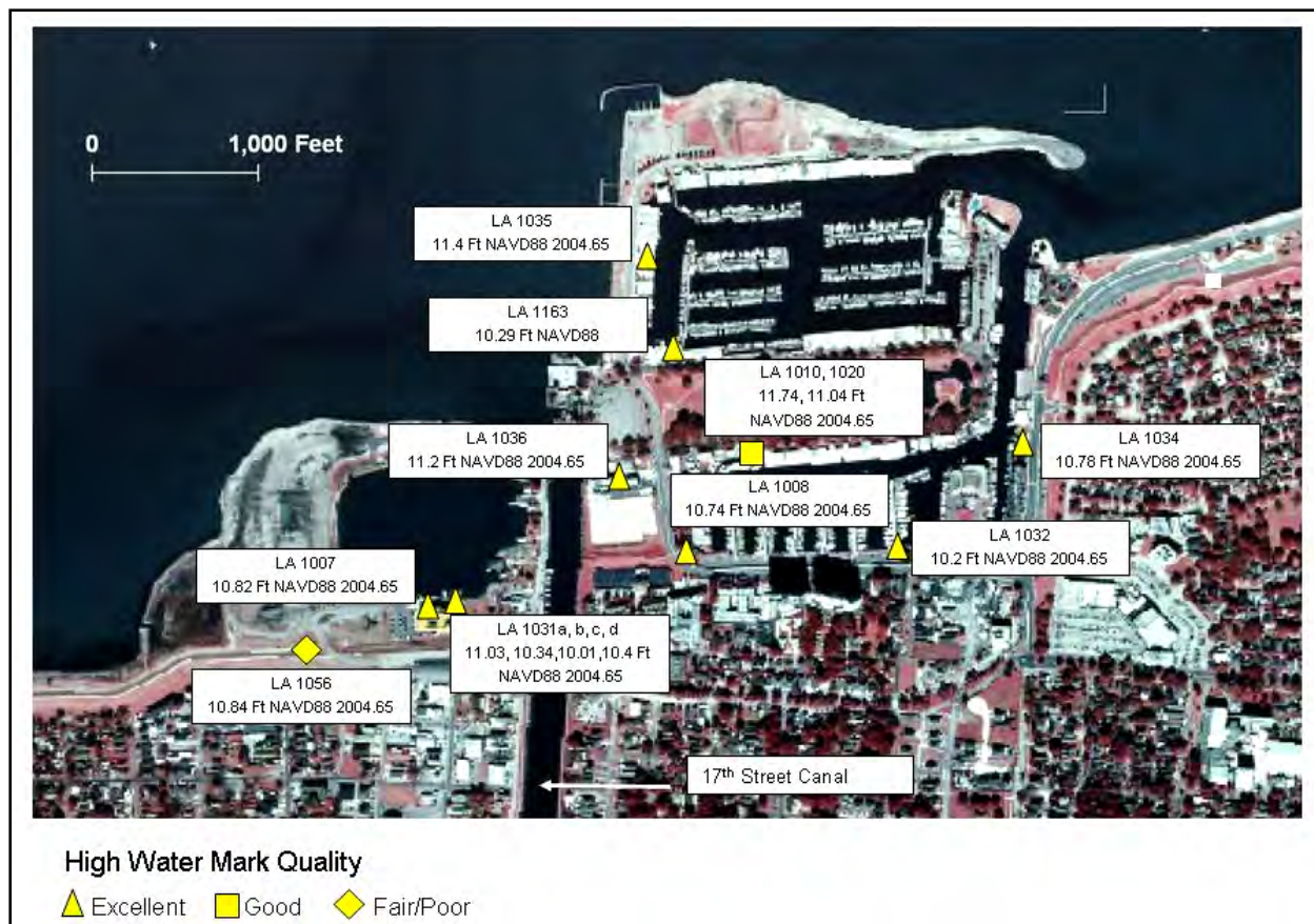
Figure V-26. High water marks on the west side of the entrance to the 17th Street Canal
