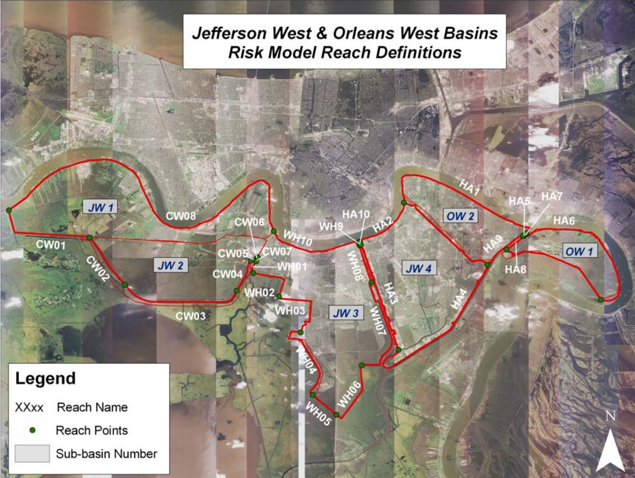
Figure 2. Orleans Parrish West bank Basin reaches (HA1,HA 5-HA9) and sub-basins (OW 1 and OW 2) definition for use in the risk model.
