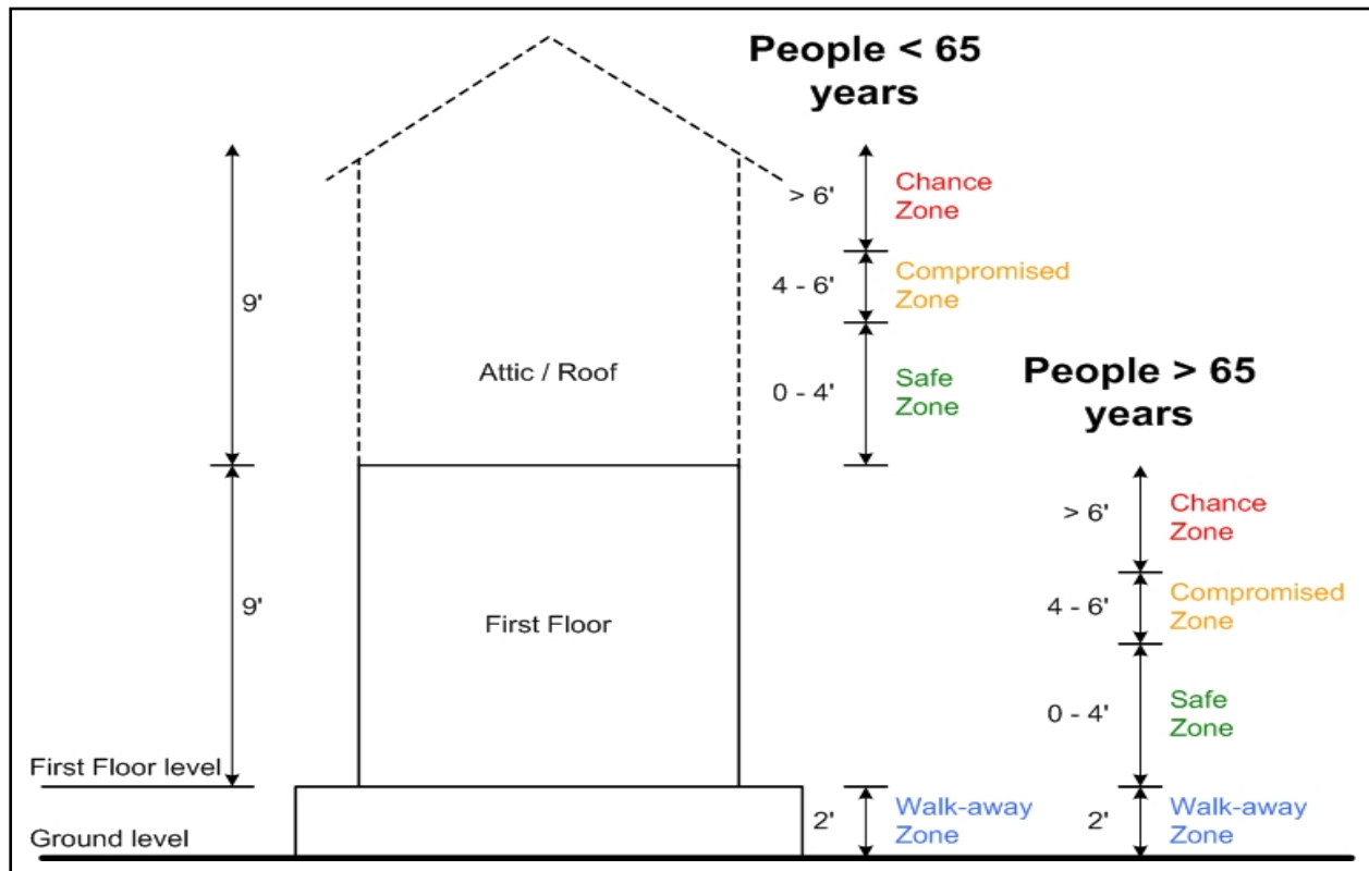
Figure 12-2. Example of LIFESim architecture and definition of zones for estimating fatalities.
