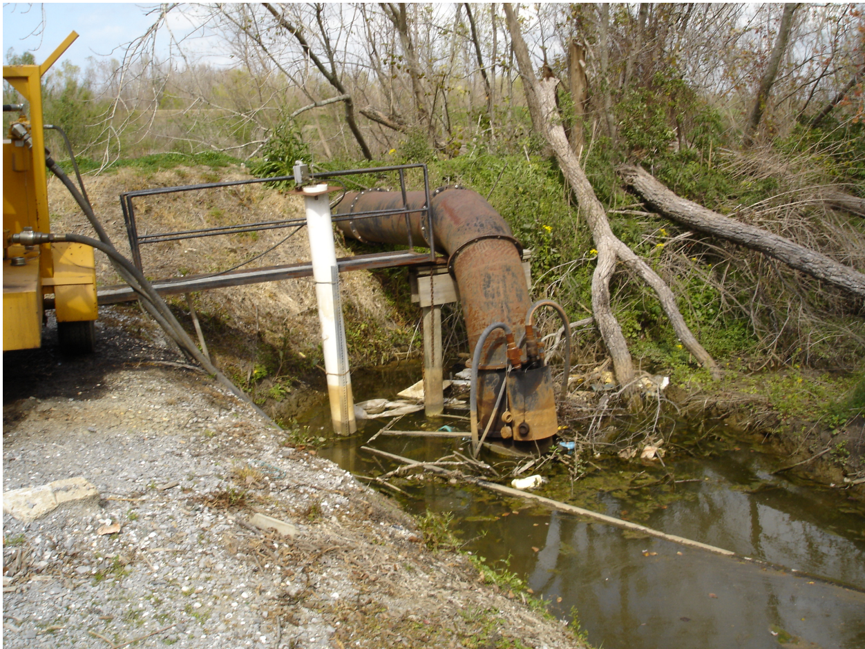
Figure 25. Hydraulically driven submersible pump.
