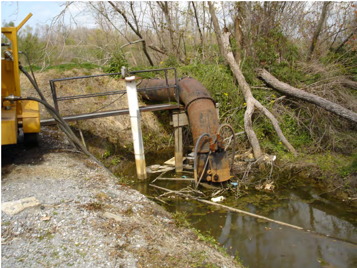
Figure 25. Hydraulically driven submersible pump.
