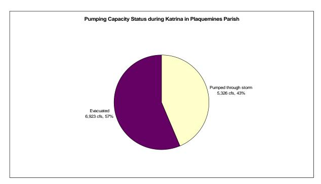
Figure 18. Plaquemines Parish pump status during Hurricane Katrina (by rated capacity).
