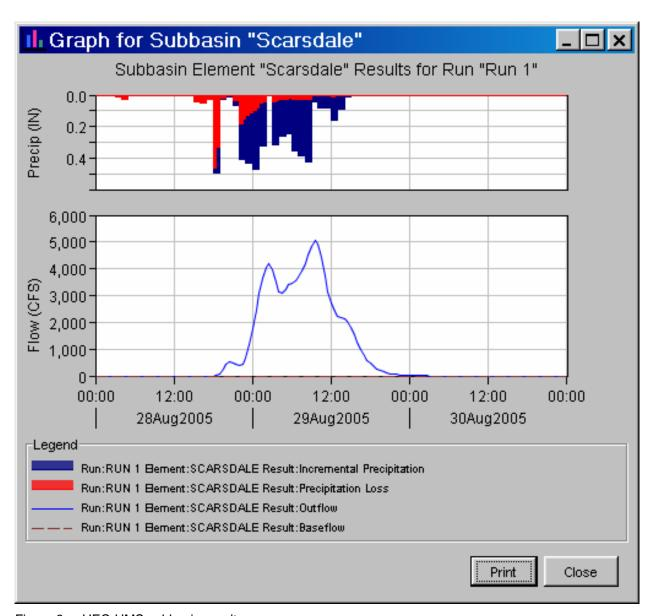
Figure 3. HEC-HMS subbasin results.
