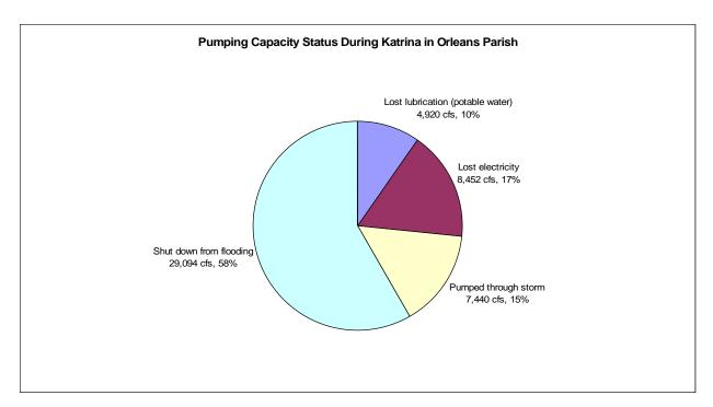
Figure 15. Orleans Parish pump status during Hurricane Katrina (by rated capacity).
