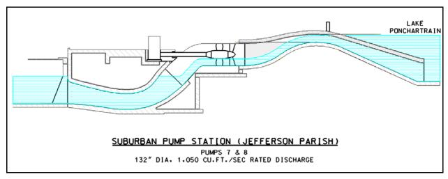
Figure 8. Graphic Representation of a pump showing reverse flow.
