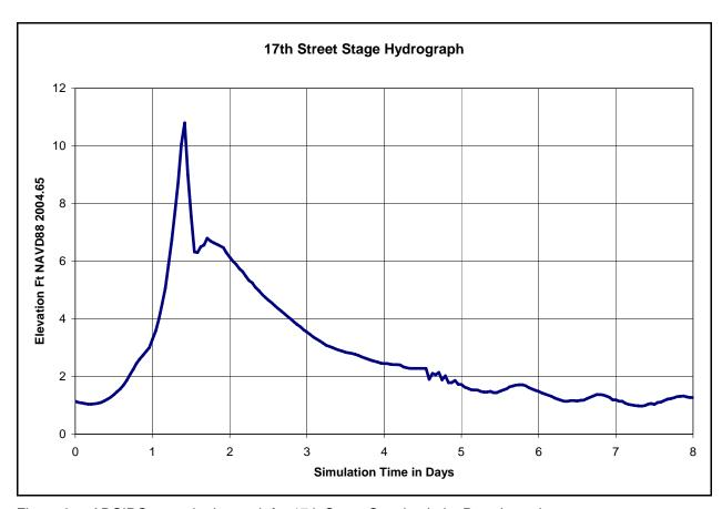
ADCIRC stage-hydrograph for 17th Street Canal at Lake Pontchartrain.
