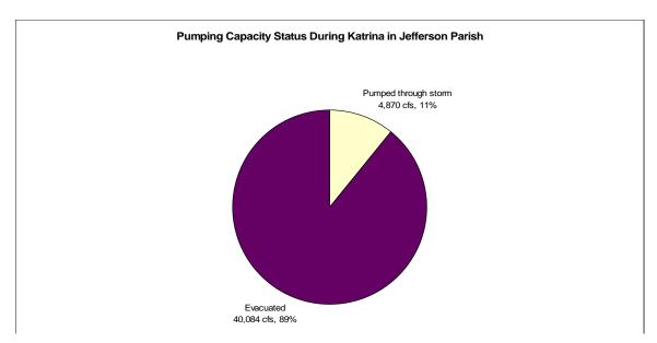
Figure 11. Jefferson Parish pump status during Hurricane Katrina (by rated capacity).
