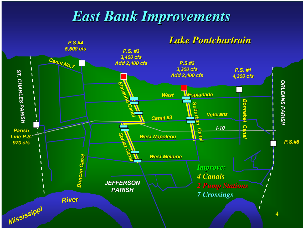
Figure 20. SELA Urban Flood Control Projects in Jefferson East Bank.
