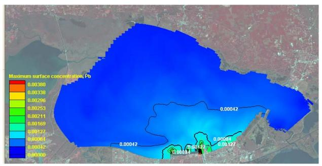
Figure 22. Maximum arsenic concentrations in the surface water layer of Lake Pontchartrain estimated using a contaminants fate model for the actual flood condition.
