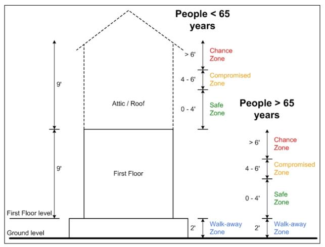
Figure 16. Modified Building Submergence Criteria
