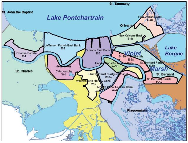
Figure 20. The hurricane flood protection system surrounding 13 sub-basins, or polders, in greater New Orleans forms the boundary between the inner and outer ecosystems of the Mississippi River delta region.
