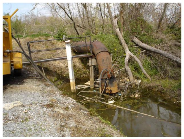
Figure 23. Hydraulically Driven Submersible Pump
