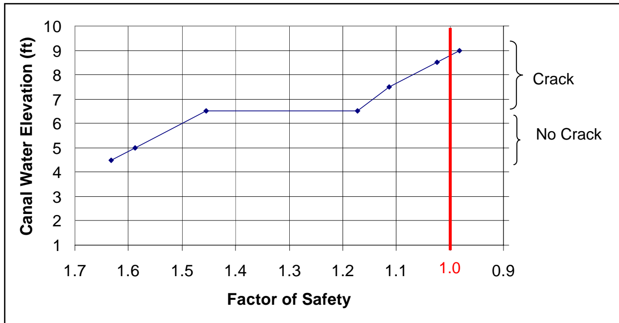
Figure 22. Factor of Safety Versus Canal Water Elevation Computed in the Soil-Structure Interaction Analysis of Station 10+00 on the 17th Street Canal East Side Breach
