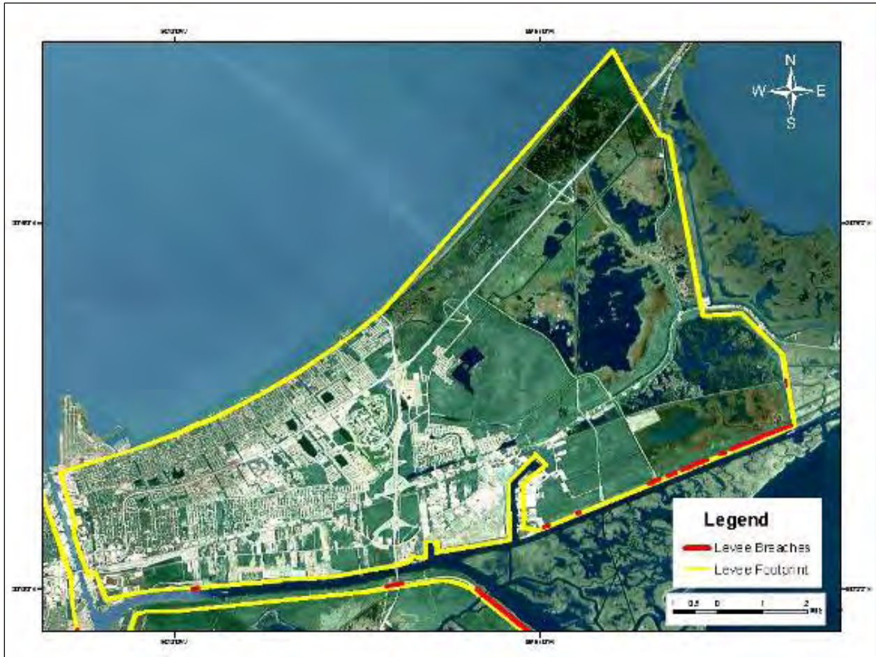
Figure 64. NOE Basin Post-Katrina Breaches
