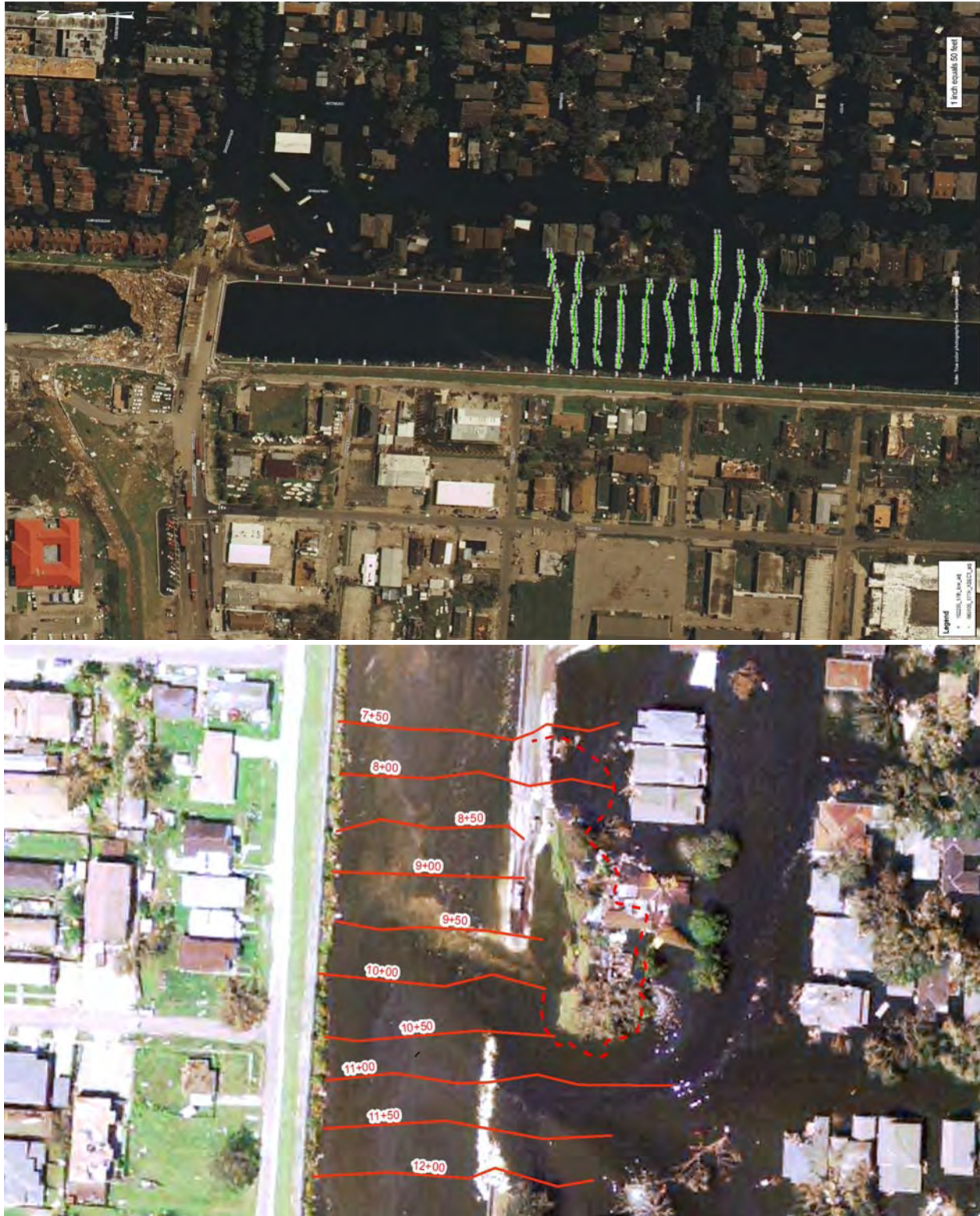
Figure 5. Location of Multi-Beam Sonar Survey Cross-Sections at the 17th Street Canal Breach
