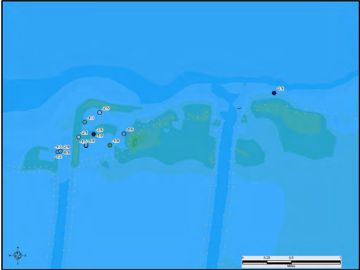
Figure 5-13e. Topographic contours (ft) and HWM elevation errors (ft) with the error value (ft). Detail of Orleans Parish and southern shore of Lake Pontchartrain
