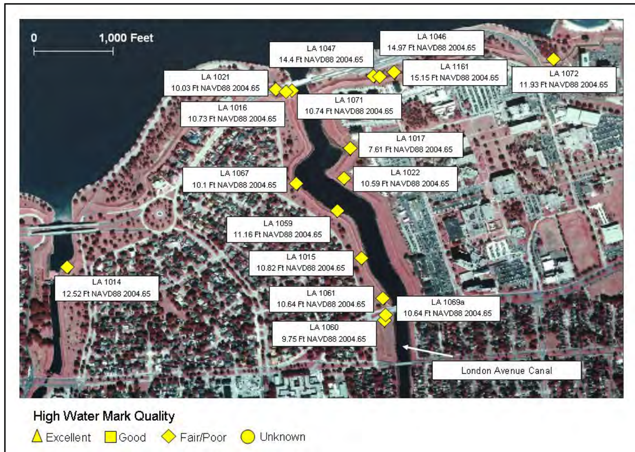
Figure 1-93. Location of high water marks near entrance of London Avenue Canal.
