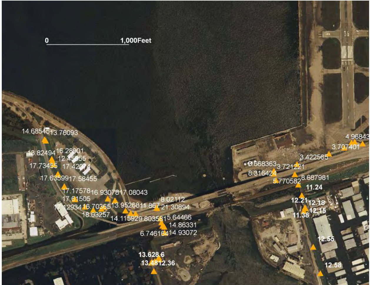
Figure 9-4. Floodwall elevations at the IHNC entrance to Lake Pontchartrain
