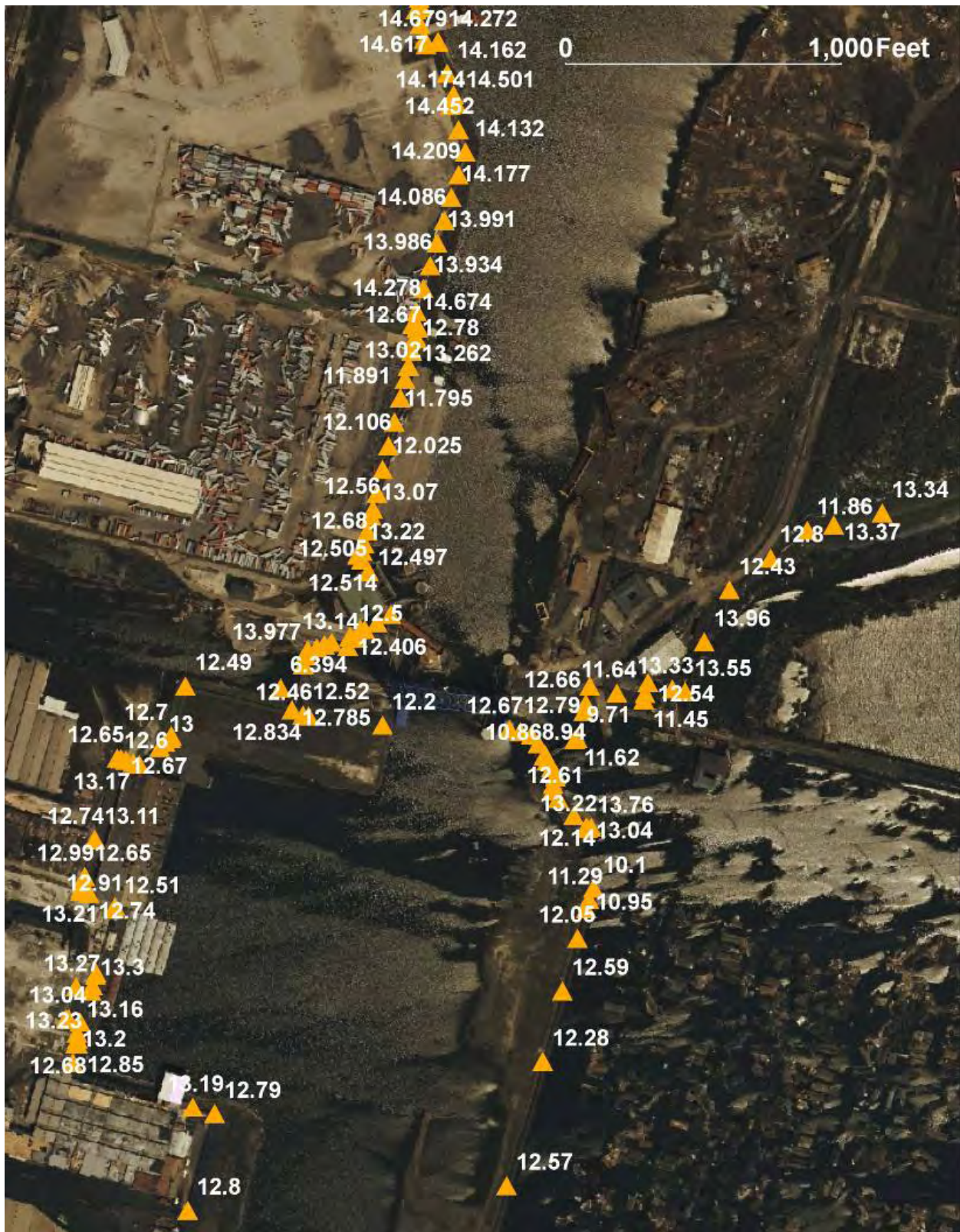
Figure 9-5. Floodwall elevations at the IHNC
