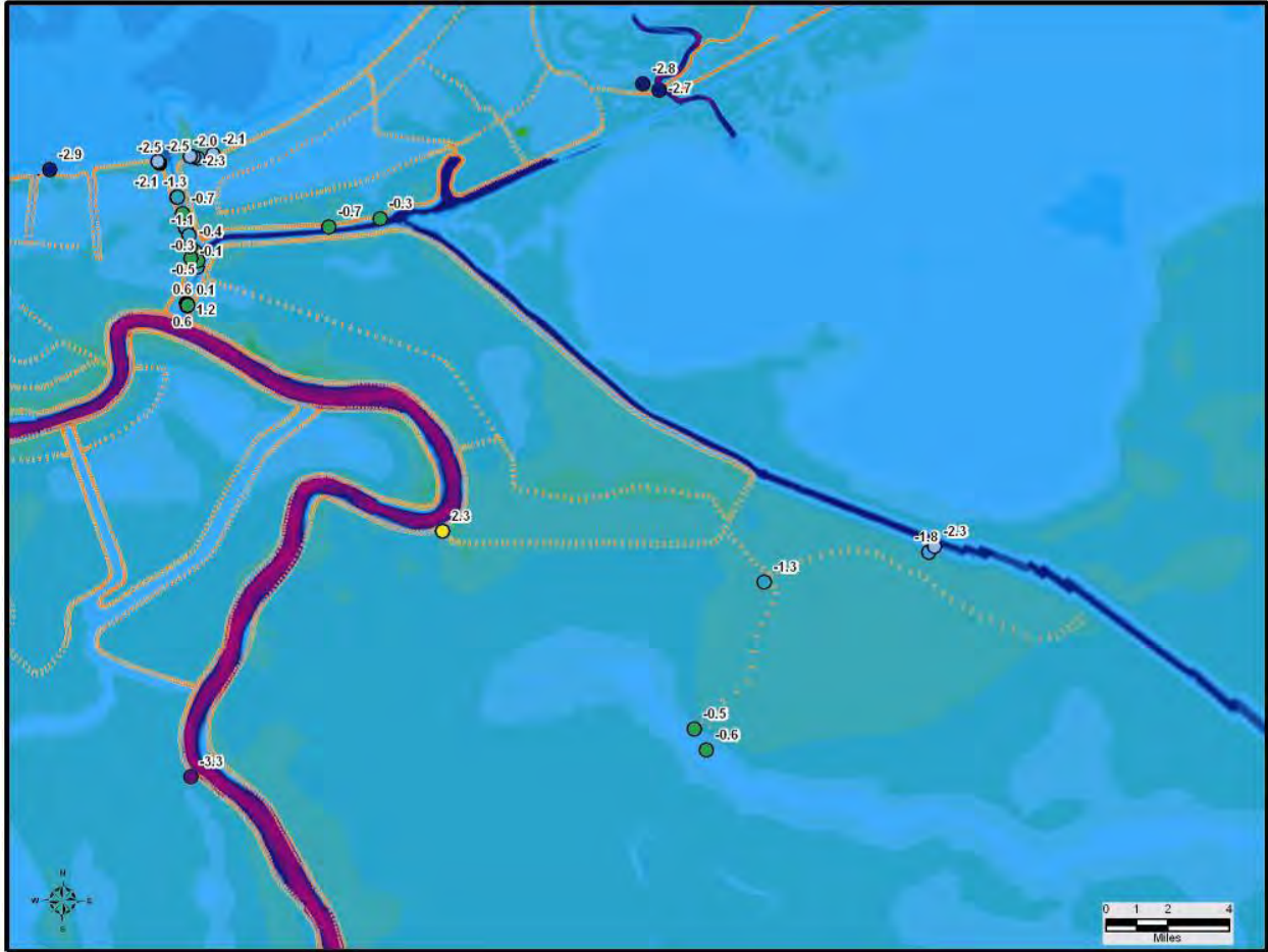
Figure 5-13c. Topographic contours (ft) and HWM elevation errors (ft) with the error value (ft). Detail in the vicinity of metropolitan New Orleans
