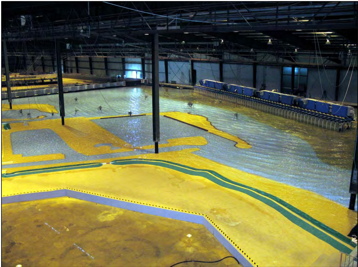
Figure 12-4. 1:50 scale model of 17th St Canal and vicinity. The directional spectral wave generator used for part of the testing is shown on the right side of the photo
