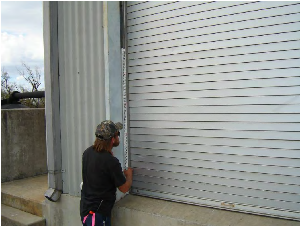
Finished Floor = 9.52 feet NAVD88(2004.65) Field Book 060852
