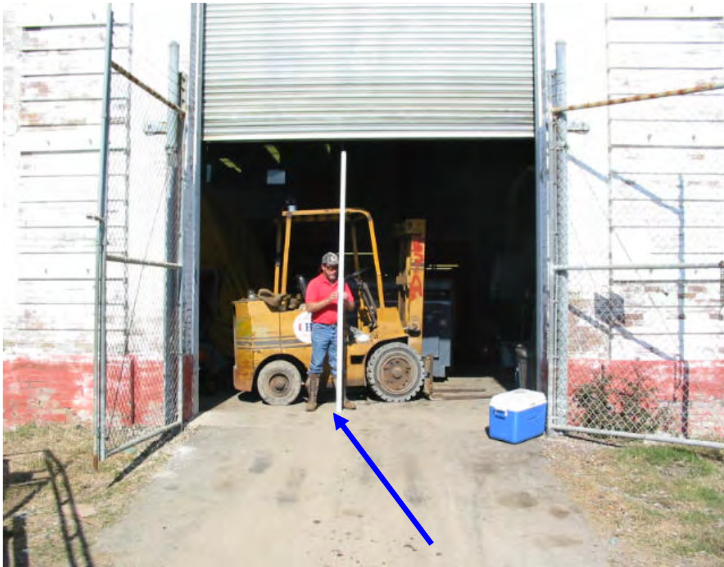
Finished Floor = 0.75 feet NAVD88(2004.65) Field book 060851
