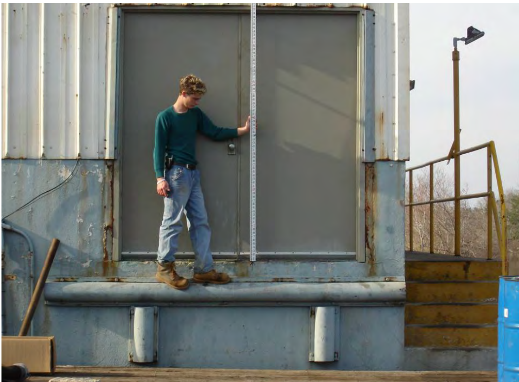
Finished Floor = 6.74 feet NAVD88(2004.65) Field Book 060854
