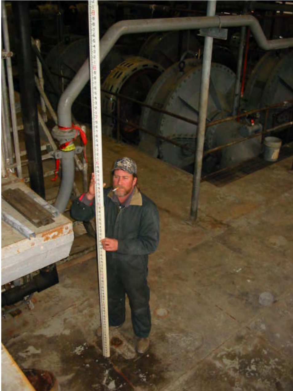
Finished Floor = 1.88 feet NAVD88(2004.65) Field Book 060851
