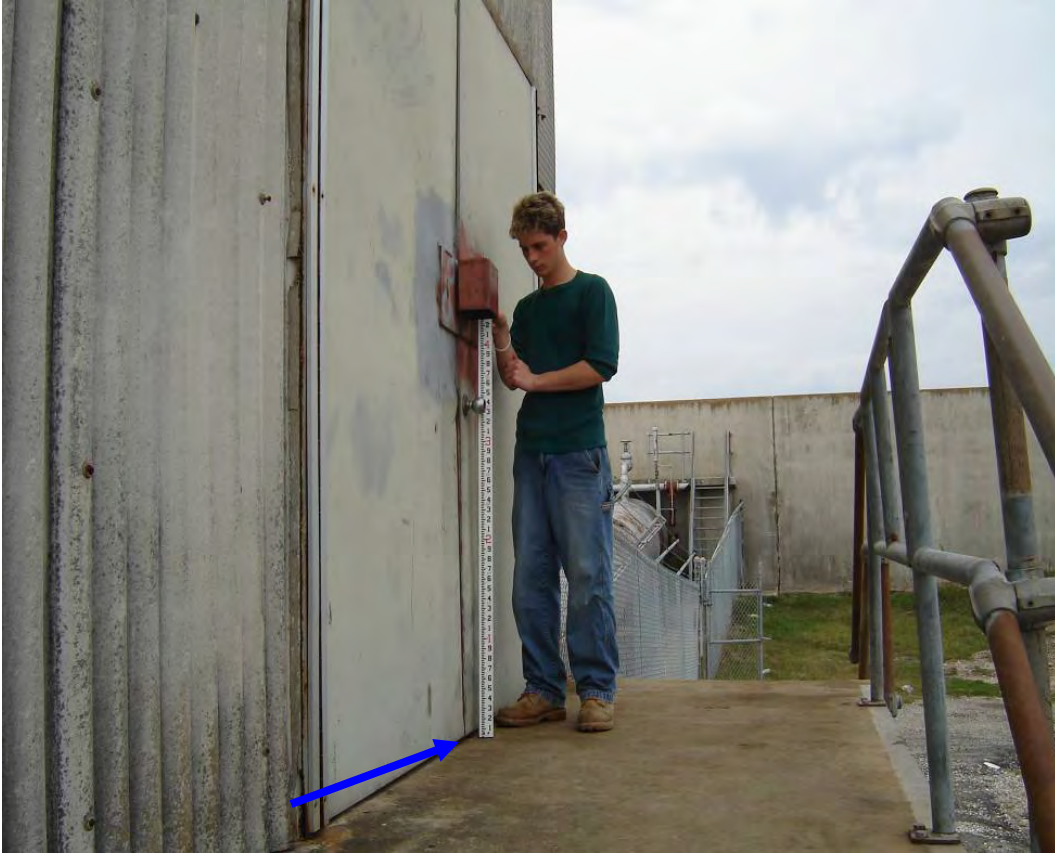
Finished Floor #2 = 9.16 feet NAVD88(2004.65) Field Book 060851
