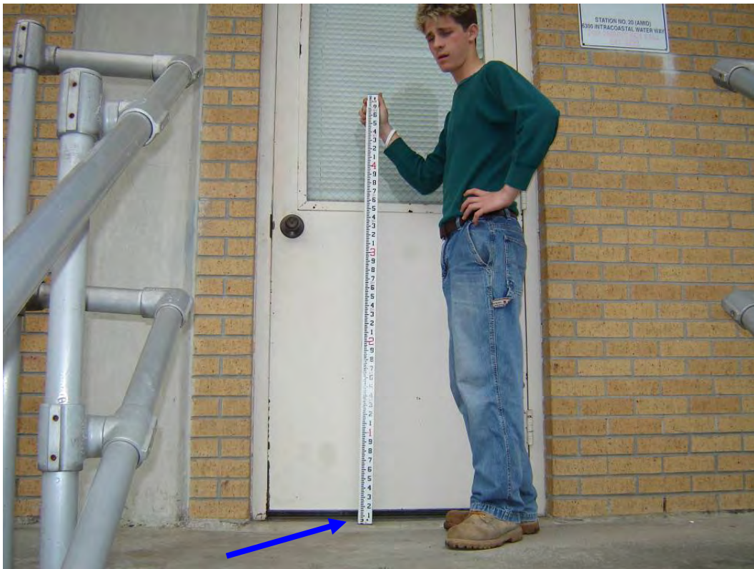
Finished Floor (Upper) = 19.20 feet NAVD88(2004.65) Field Book 060851
