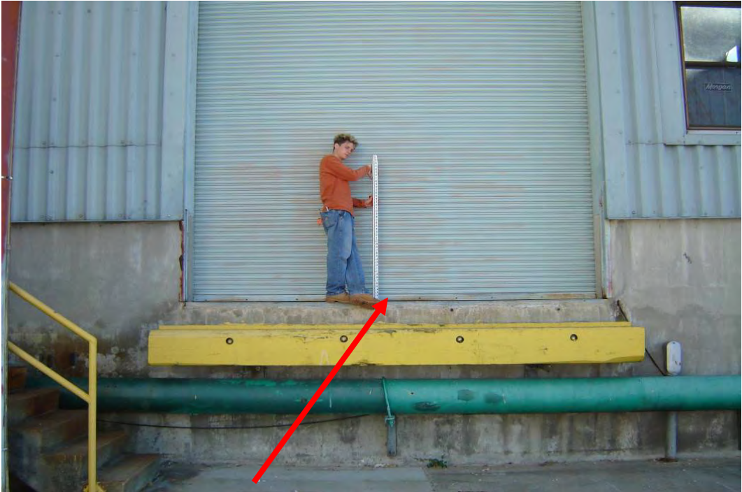
Finished Floor = 2.11 feet NAVD88(2004.65) Field Book 060852
