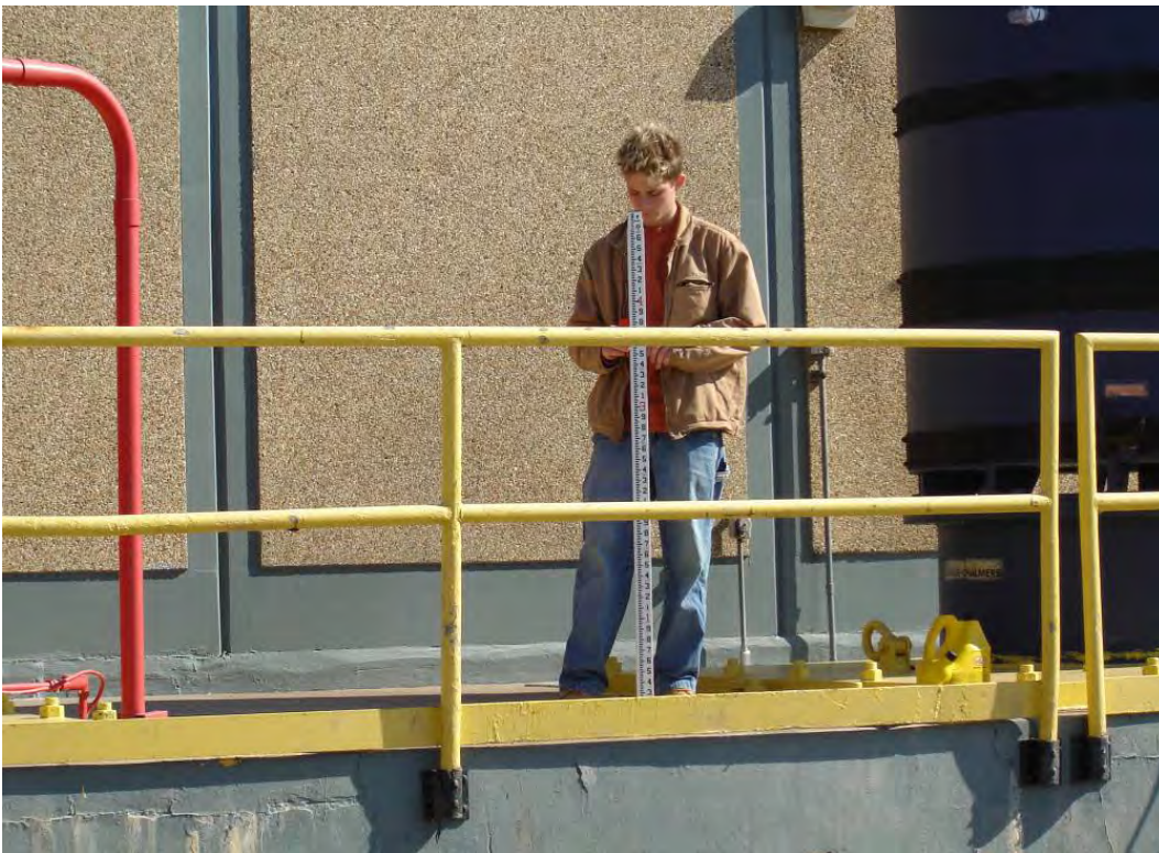
Finished Floor = 3.15 feet NAVD88(2004.65) Field Book 060852
