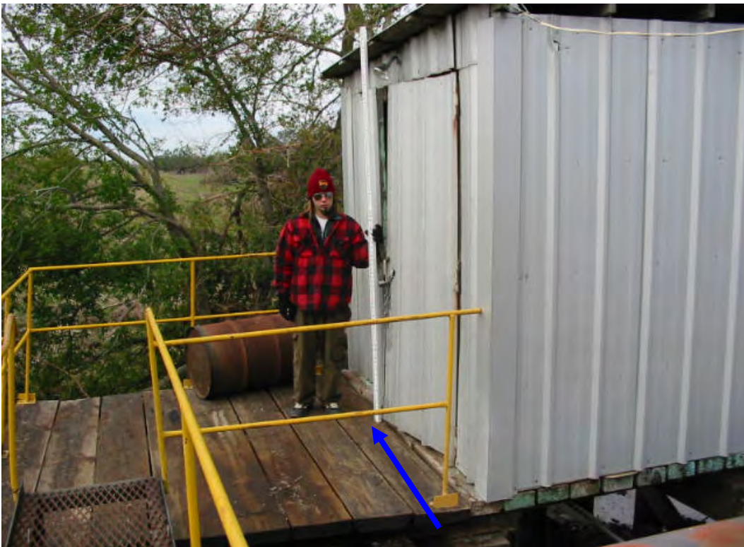
Finished Floor #2 = 8.11 feet NAVD88(2004.65) Field Book 060852
