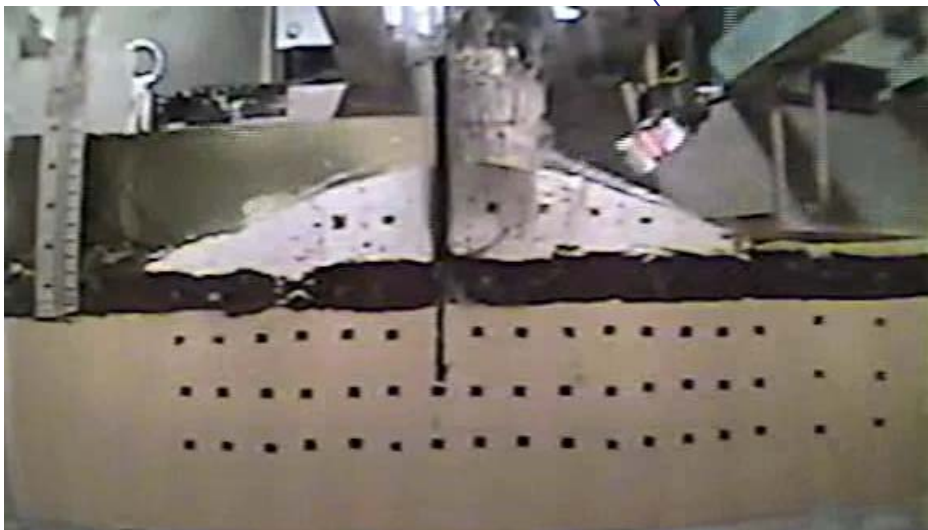
Crack opening phase, marked by start of wall rotation and pore pressure rise around the toe of the sheet pile (ERDC London South)
