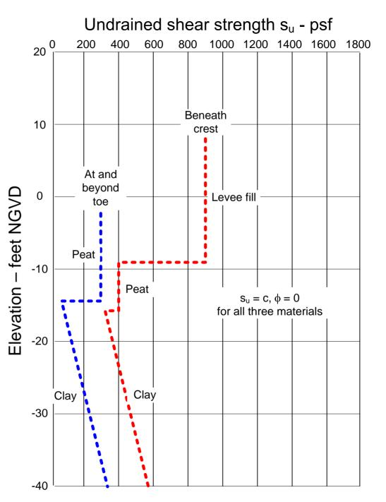
Comparison of IPET shear strength model with design shear strengths
