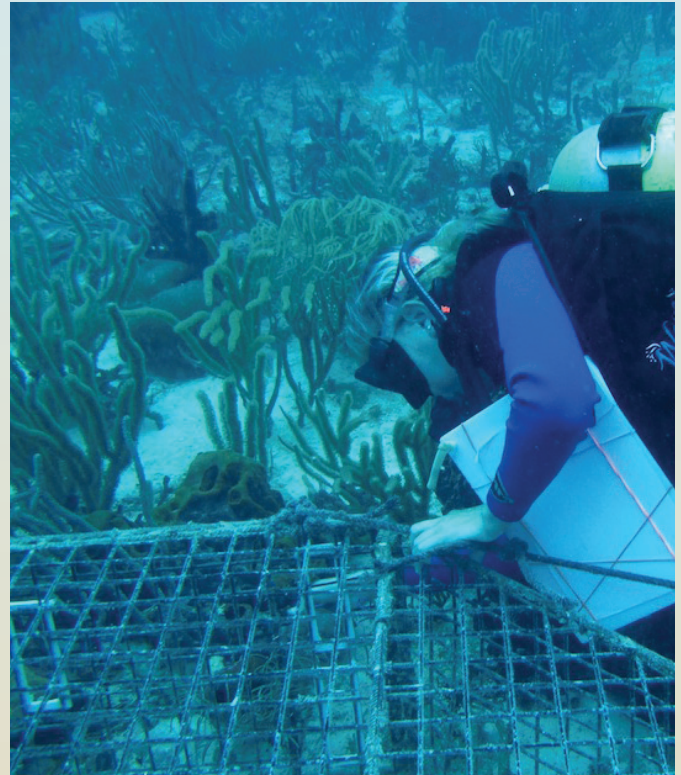
SEFSC scientific divers installing prototype vented traps in the USVI. Photo credit: Vanessa Wright.
