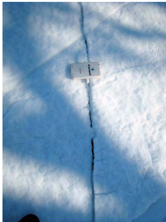
Figure 5.14 Ice Crack Running Parallel to Shore (March 2008)
