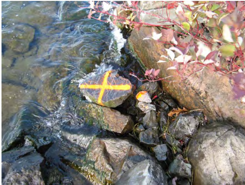
Figure 4.4 Typical Marking of Rip-Rap Stone
