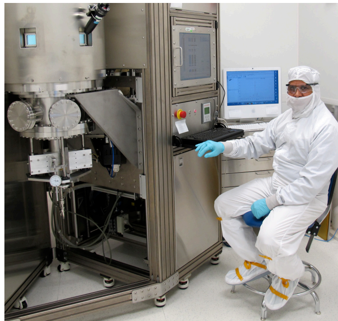
CNM scientist Anirudha Sumant produces ultrananocrystalline diamond (UNCD) films, promising for applications in communication, biomedical devices, and tribology, using a microwave plasma chemical vapor deposition system installed in the CNM clean room.
