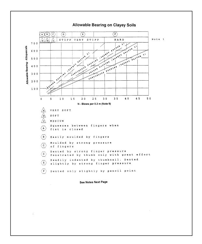
Allowable Bearing on Clayey Soil Figure 9-5.2b
