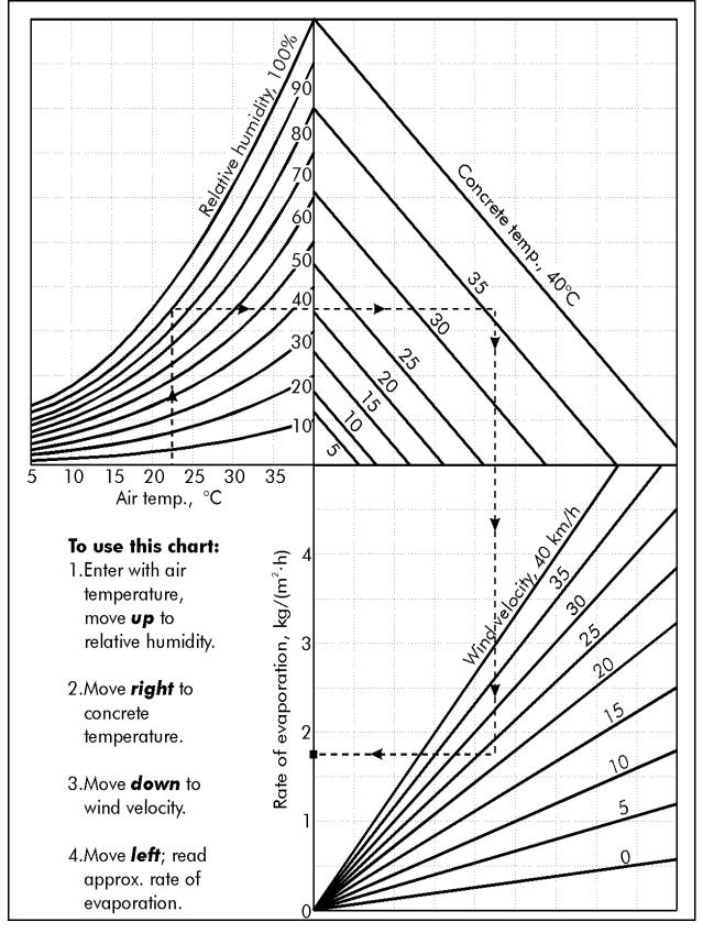
Note: Example shown by dashed lines is for an air temperature of 22.5°C, relative humidity of 90 percent, concrete temperature of 36°C, and a wind velocity of 22.5 kilometers per hour. This results in a rate of evaporation of 1.75 kilograms per square meter per hour.
