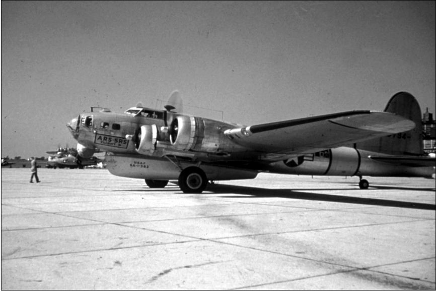
A lifeboat can be seen fitted to the underside of this SB-17G.
