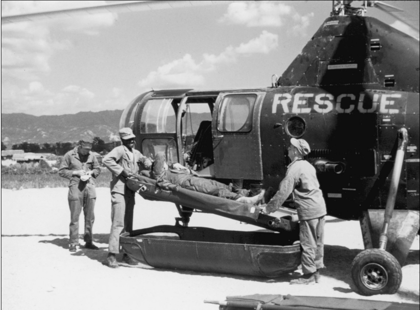
Rescue personnel load an injured servicemember into the H-5 helicopter's outboard capsule before transferring him to a medical facility.
