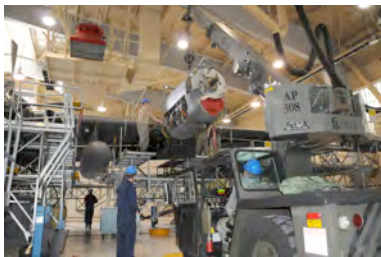
Installation of a C-130 engine
