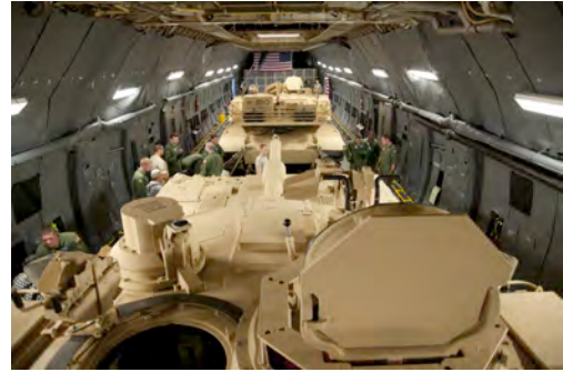
Two M-1 Abrams tanks are loaded in the cargo area of a C-5M Super Galaxy
