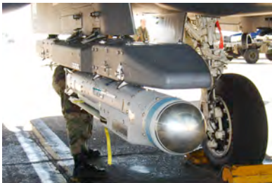
GBU-53B loaded on an F-15E
