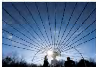
Sweeping dipoles on a Solar Radio Spectrograph
